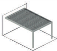
Pared Portería Lama Paralela a Pared On facade Louvers parallel to the wall
